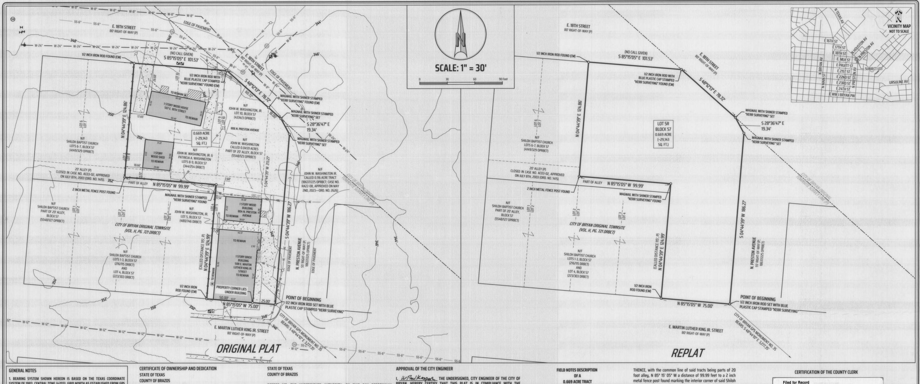
SYSTEM OF 1983, CENTRAL ZONE (4203), GRID NORTH AS ESTABLISHED FROM GPS OBSERVATION USING THE LEICA SMARTNET NAD83 (NA2011) EPOCH 2010 MULTI-YEAR CORS SOLUTION 2 (MYCS2).
